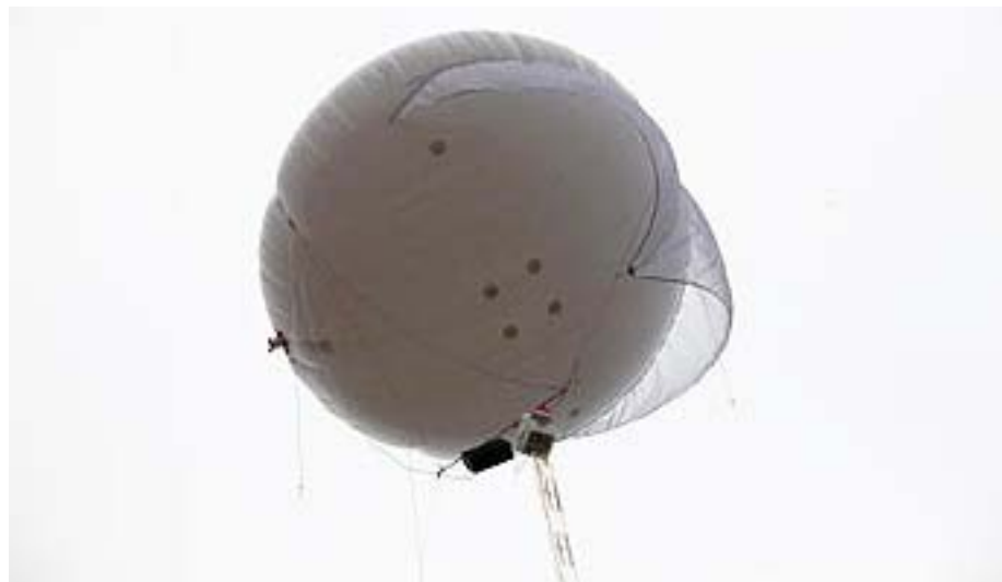
A latex helium-filled weather balloon and radio transmitting component from the Combat SkySat System floats tethered above the 21 area parade deck. When launched into the air and sustained at 65,000 to 100,000 feet, the system covers a range of 460 to 700 miles.
